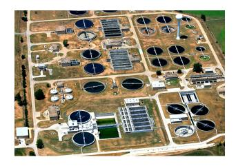
Municipal water resource recovery refers to the physical, chemical, and biological processes to remove pollutants and nutrients from wastewater before discharging into a waterbody.
