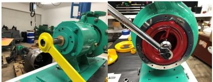
• Remove the cutter bar, Suction plate O-ring and impeller from the pump.
