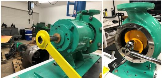
• Install the cutter bar and suction plate O-ring. Note the orientation of the "X". It will need to be located at the 12:00 position. Use a small amount of grease or anti-seize may be needed to help hold the O-ring in place.
