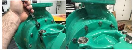
• Once the suction manifold is removed, using the shaft holding tool loosen and remove the cutter nut.
