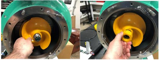
• Using the shaft holding tool, torque the cutter nut to 50 ft/lbs.
