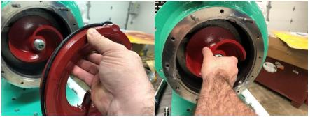
• Replace the impeller, cutter bar and cutter nut with the opposite-colored parts.
